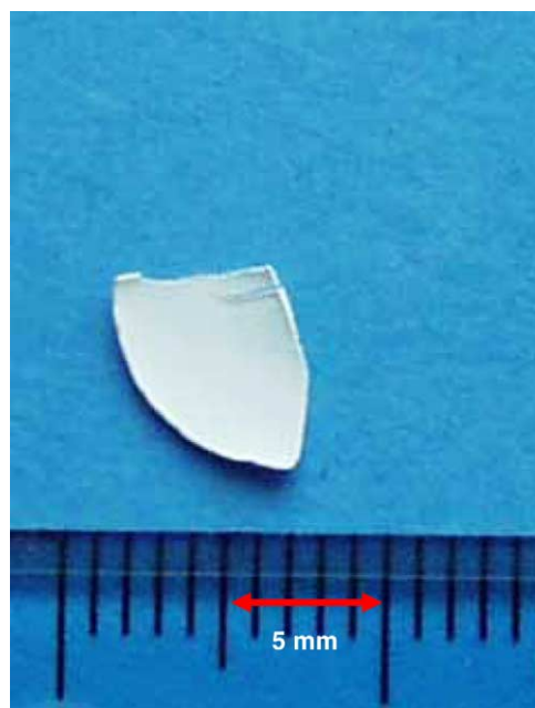
Fig. 2. Photograph of three dimensionally ordered macroporous Li–La–Ti–O ceramic calcinated at 600\ ^\circ\text{C} .
